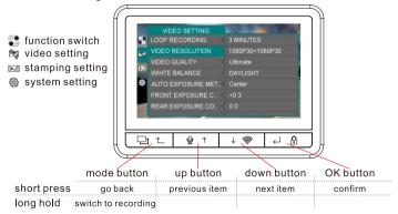
For setting details, please check the SETTING section at page16. Press and hold MODE button again will go back to recording mode.
